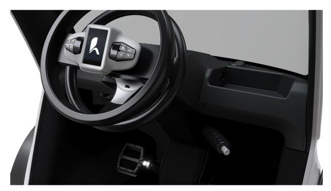
Figure 22: Parking brake in parking position
