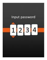
If you have activated the password protection, the system asks for it before each start of the hopper. In the input window you can enter each Enter the first digit of the password using the "Up" and "Down" commands. By means of the "Confirm" command you will move from one digit to the right to the next. The menu closes automatically after you "Confirm" the entry of the fourth digit. -' Chap. 2.5.3 "Opening and navigating the master menu", p. 18
