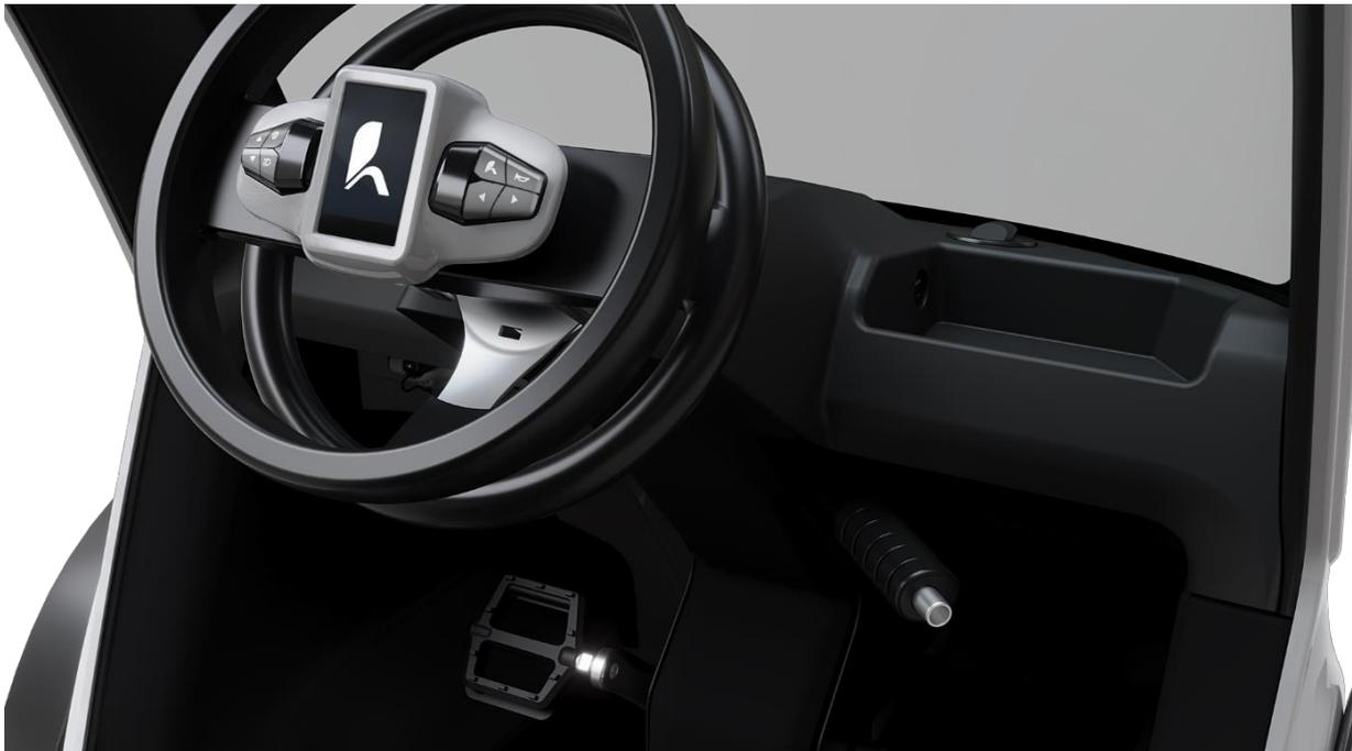
Figure 22: Parking brake in parking position
