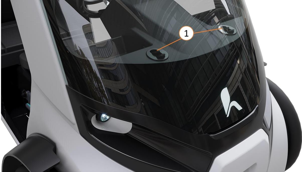
Figure 7: Position fan heater
