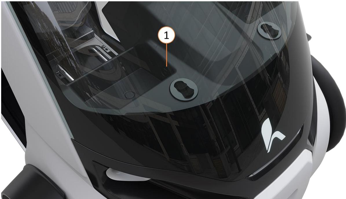
Figure 6: Position USB ports
